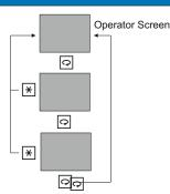
While in normal operation state, upper display displays the remaining time, lower display displays the remaining time of second timer. This view is called Operator-Screen.
