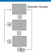
While in normal operation state, upper display displays the remaining time, lower display displays the remaining time of second timer. This view is called Operator-Screen.
