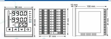
Panel Cutting Dimensions =  $92 \pm 0.5 \text{ mm} \times 92 \pm 0.5 \text{ mm}$
