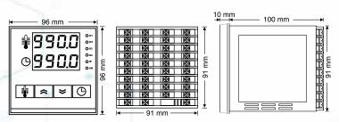
Panel Cutting Dimensions = 92 ± 0,5 mm x 92 ± 0,5 mm
