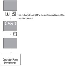
In order to access the operator page parameters, the and keys are pressed together while the vice is energized, the LHn. I parameter appears on the screen. Password must be entered here, if any, otherwise the factory setting is defined as "0".
