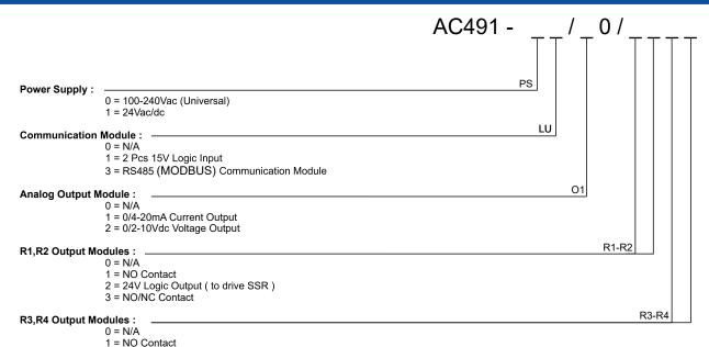
Note: If R1 relay is coded as 3 (NO / NC), and relay R2 is selected as contact, it must be coded as NO / NC.
